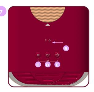
Press one of the buttons **C-D-E** and wait for the machine to complete the water filling cycle. Indicator **B** will turn off.
