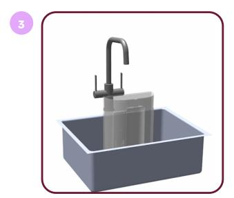
Fill the tank with fresh, non-carbonated water. Never exceed the maximum level indicated in the tank.
