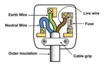
The toaster must be earthed. Fit a 13A BS1362 fuse in a 13A BS1363 plug. Fit the green/yellow wire to E, the blue wire to N and the brown wire to L. Fit the cord grip. If in doubt, call an electrician. Don't use a non-rewireable plug unless the fuse cover is fitted. If you remove the plug, dispose of it.
