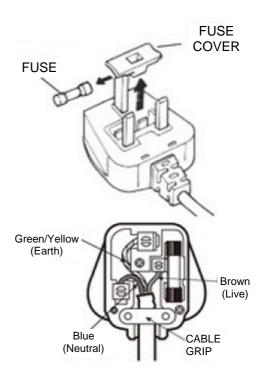
As the colours of the wires in the mains lead may not correspond with the colour markings identifying the terminals in your new plug, proceed as follows:
